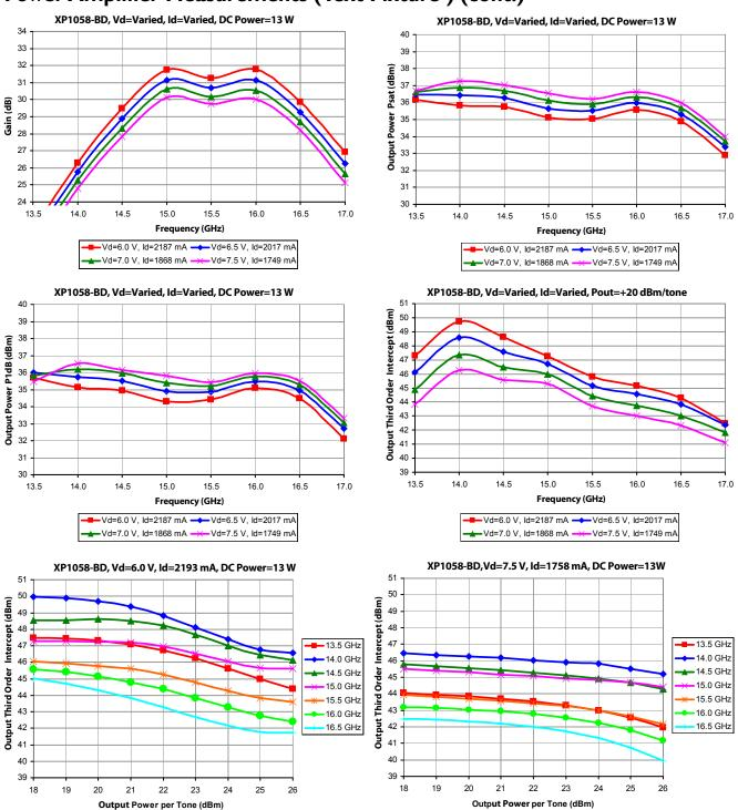
Note [1] Measurements – Test Fixture data includes all bond wire parasitics, uncompensated RF In/Out Mimix T-Pad transitions and RF ceramic circuit losses. For Gain and Output Power curves RF In/Out circuit losses have been removed.
