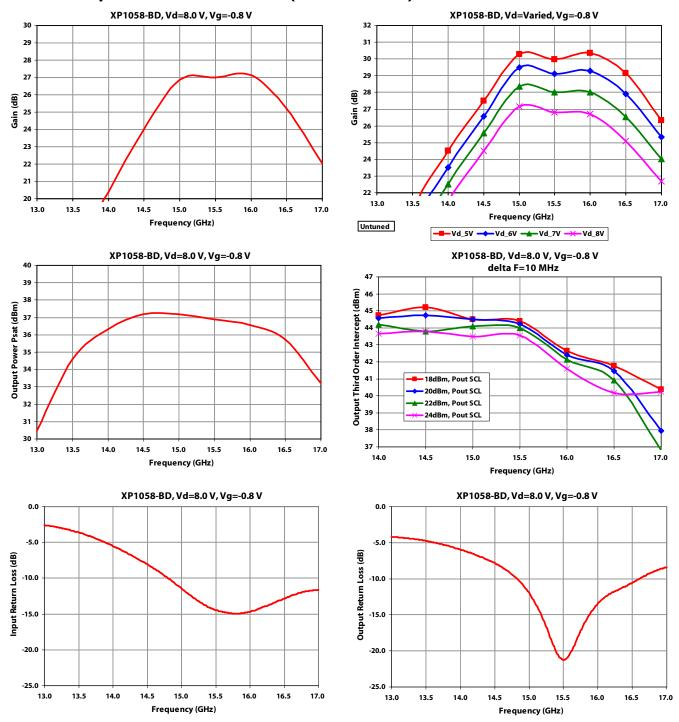
Note [1] Measurements – Test Fixture data includes all bond wire parasitics, uncompensated RF In/Out Mimix T-Pad transitions and RF ceramic circuit losses. For Gain and Output Power curves RF In/Out circuit losses have been removed.
