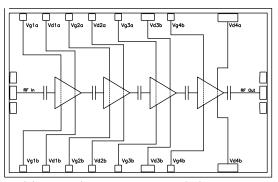
performance and most reproducible results. Depending on the supply voltage available and the power dissipation constraints, the bias circuit may be a single transistor or a low power operational amplifier, with a low value resistor in series with the drain supply used to sense the current. The gate voltage of the pHEMT is controlled to maintain correct drain current compensating for changes over temperature.
